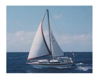
Manufacturer Reinke Year 1990 Designer Reinke Sail or Power Sail New or Used Used Hull Type MonoHull Hull Material Steel LOA 43 Beam 12 LOD 42 Draft 8 LWL 40 Sail Area 93 Displacement 13
